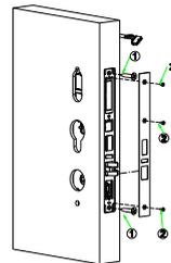
6: 对准孔位分别如下图装入长方轴和短方轴
